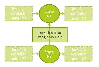
Variables associated with tasks: Ws<sub>trasfer,n</sub>- binary variable Wf<sub>trasfer,n</sub>- binary variable Bs<sub>trasfer,n</sub>- batch size variable Bp<sub>trasfer,n</sub>- batch size variable Bf<sub>trasfer,n</sub>- batch size variable Tf<sub>trasfer,n</sub>- timing variable
